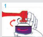
To install the horn, you need to screw it on the pressurised container
