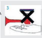
The signal horn must always be used in upright position
