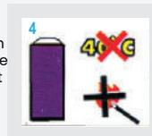
Do not store the pressurised container in direct sunlight. Do not expose to sunlight for very long hours or to temperatures exceeding 40 °C. Do not pierce or burn after use.
